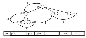
Figure 6.1: The JavaScript program P0 performs 3 function calls, P01, P02, and P03, and P01 performs two function calls, P011 and P012. Thus, we have created a speculation tree. If we traverse this tree from left to right, we get the same function call order as in a sequential execution, i.e., P0, P01, P011, P012, P02, and finally P03. We denote this order as *function\_order*.
