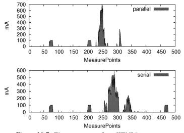
Figure 10.7: The power usage for a HTML5 use-case.
