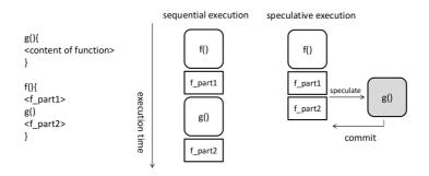
Figure 1.3: A schematic of the workings of Thread-Level Speculation.
