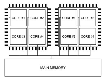
Figure 1.1: An example schematic of a dual-quadcore architecture with two CPUs which contain 4 cores each, however all cores have access to the same memory. It is usually up to the programmer to take advantage of the cores.
