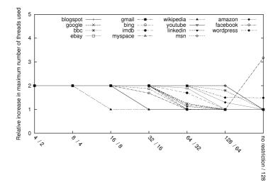
Figure 7.11: The relative increase in the highest number of concurrent threads increasing the maximum number of threads from 2 to 4, 4 to 8, 8 to 16, 16 to 32, 32 to 64, 64 to 128 and 128 to no limitation.
