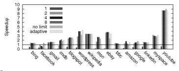
Figure 8.5: The speedup when we limit the checkpoint depth to 1, 2, 4, 8 and put no restriction on the checkpoint depth and the speedup of the adaptive heuristic.
