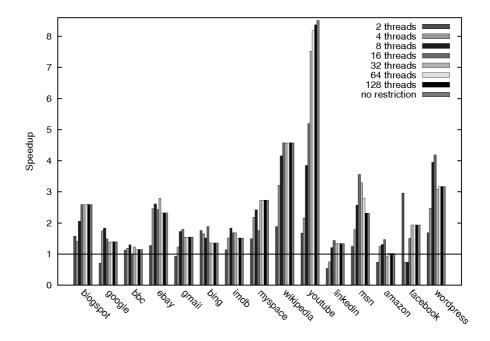
Figure 7.10: The speed up when we limit the number of threads to 2, 4, 8, 16, 32, 64, 128 and with no restriction on the maximum number of threads (average speed up, excluding the *Youtube* use case is 2.09).
