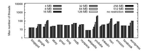
Figure 7.8: The largest number of threads when we limit the available memory to 4, 8, 16, 32, 64, 128, 256, 512MB and with no restriction on the memory usage.
