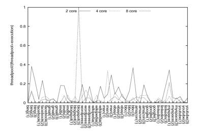
Figure 9.11: The thread pool initialization time as propotion of the total execution time.
