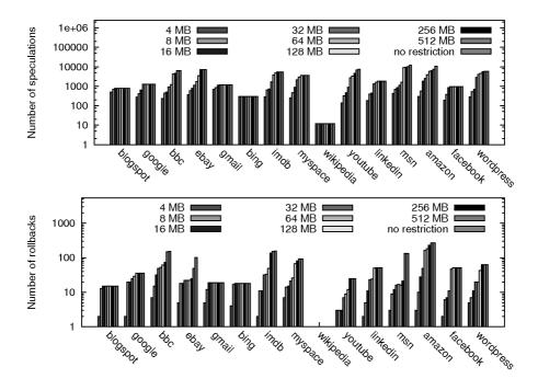
Figure 7.9: The number of speculations (upper) and the number of rollbacks (lower) when we limit the memory usage to 4, 8, 16, 32, 64, 128, 256, 512MB and with no restriction on memory usage.
